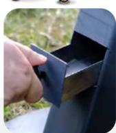
The ash formed during combustion fills the ash pan at the front of the product. It leaves very little ash. It is sufficient to empty it once in 5-6 hours.
